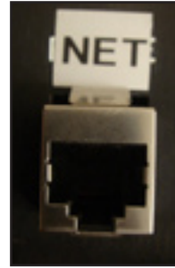
Network Connection on Laptop Plate
